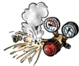
Carefully check the connection between the regulator and the cylinder valve outlet
