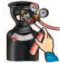
Test for leaks with leak detector solution
