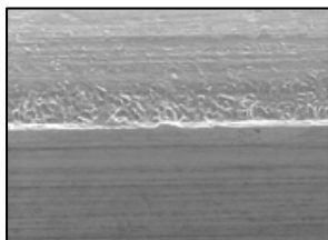
LOWER QUALITY WIRE SURFACE MAGNIFIED 60x
